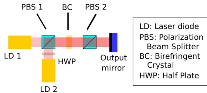
Figure 1. Schematic diagram of the rectified polarization coupling (RPC) technique for two diodes.
