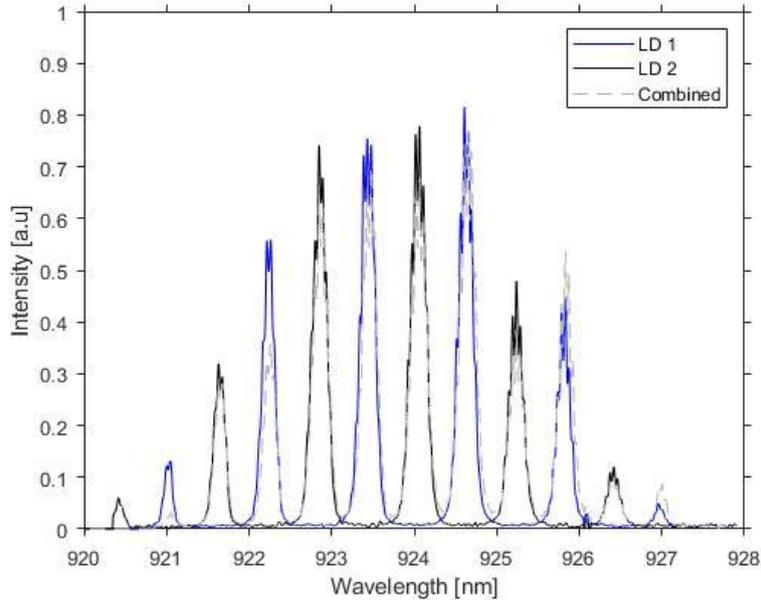
Figure 2. Experimental spectrum of two lasers combined by RPC.
