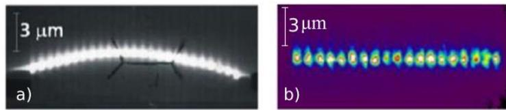
Figure 4. a) Enlarged picture of a soldered diode laser bar with a 'smile' of approx. 2  $\mu\text{m}$ . Image taken from Ref. 8. b) Enlarged picture of a diode laser bar mounted with *Clamping™*, showing a smile under 0,1  $\mu\text{m}$ .
