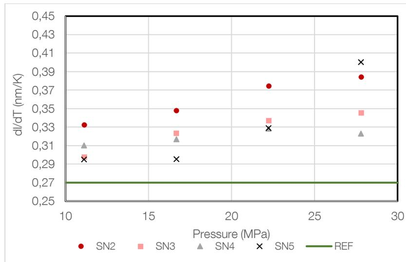
Figure 4 Wavelength tuning coefficient as function of the uniaxial load of four laser modules set at a pre-load of  $11.2\text{N/mm}^2$ . The solid green line sets the reference for this kind of semiconductor.
