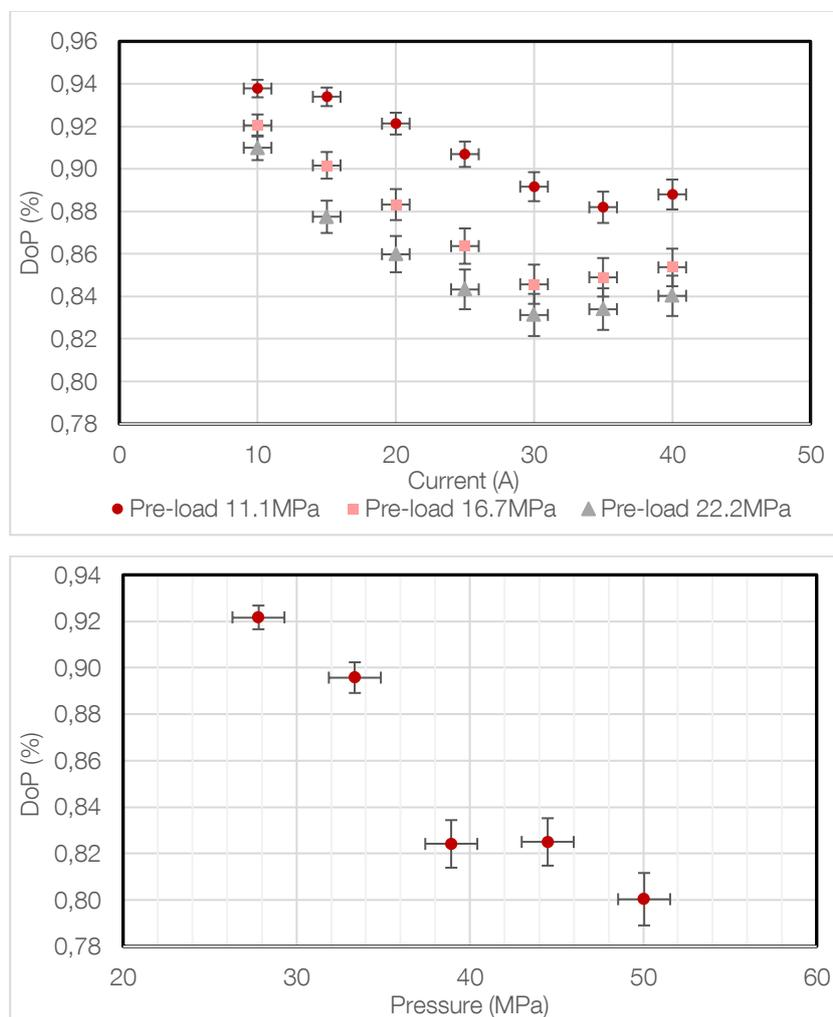
Figure 2 Degree of TE-polarization of (a) a laser (labelled SN2) bar under constant uniaxial stress along the [001] axis as function of the CW driving current and (b) another laser module (labelled SN3) at a constant driving current  $I=40\text{A}$  as a function of the load
