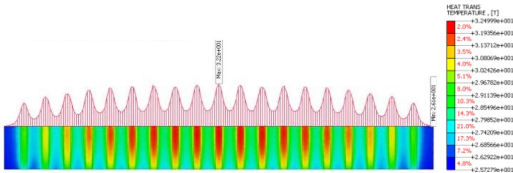
Figure 6 Thermal simulation of the laser bar under study performed with MidasNX. The thermal contact between the bar and the heatsink is assumed ideal. The laser bar has been modeled as a solid block of GaAs, 40W of heat being generated homogenously among 19 emitters directly in the interface between the bar and a pure Cu heatsink.
