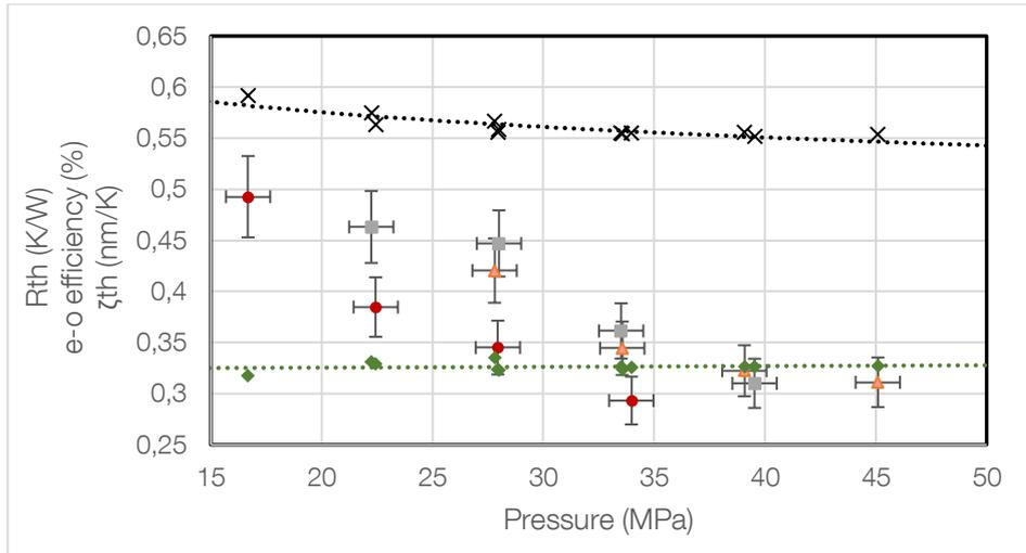
Figure 5 Thermal resistance as function of the uniaxial force applied. The three different series account for different pre-loads. Red circles are obtained with a pre-load of 16.67MPa, grey squares with a pre-load of 22.24MPa and pink triangles with a pre-load of 27.80MPa. Black crosses plot the electro-optical efficiency of the laser module. Green diamonds plot the wavelength tunability coefficient. Dotted lines are only eye guides.
