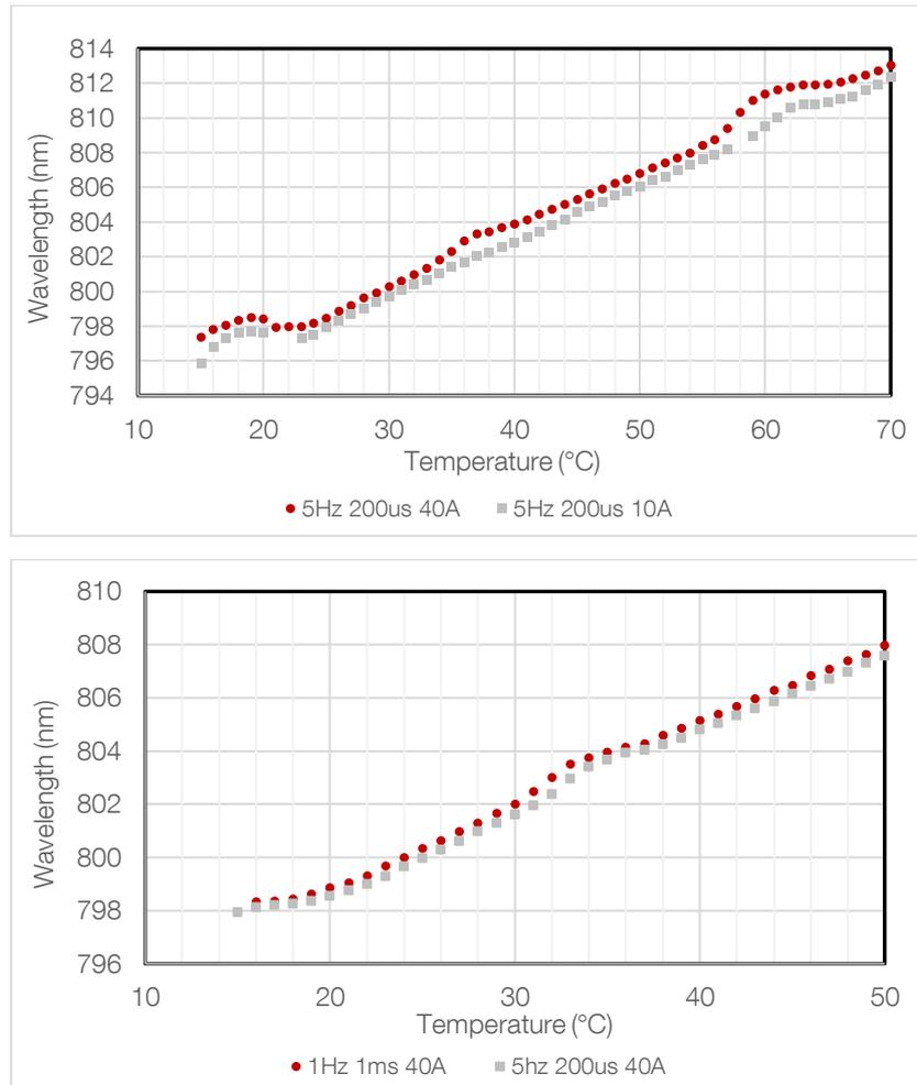
Figure 3 Wavelength tuning for different operating conditions. (top) compares the behavior when pre-load is set at 11.1MPa and the load is 0cN·m for driving currents of I=10A and I=40A while (bottom) compares pulse durations of  $t_p=200\mu s$  and  $t_p=1ms$  when the pre-load is 22.2MPa and the load is 0MPa
