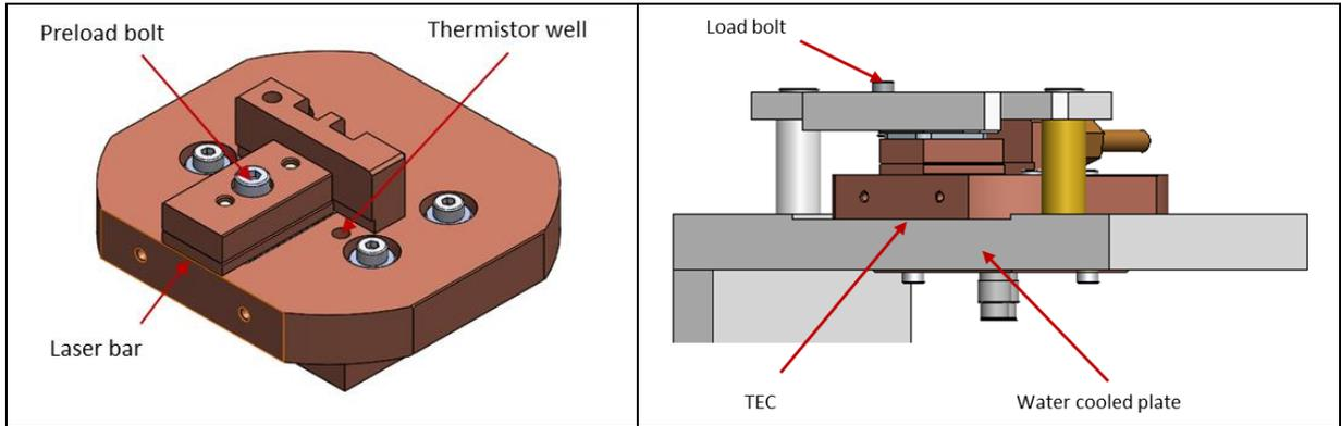
The pre-load and load forces are applied by means of screws and can be calculated from the following equations respectively:
